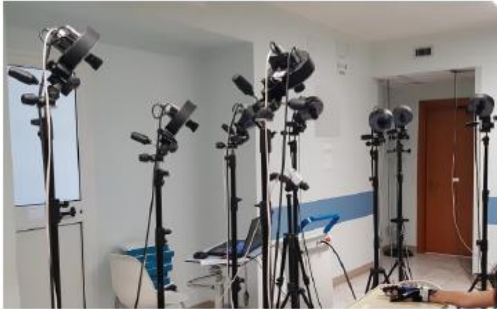
Fig. 2. Experimental Setup for the Gloreha Sinfonia glove calibration.
